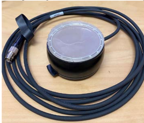
Figure 5. Coupling pad with imbedded rim, mated to transducer. Note that the air bubbles seen between the gel pad and transducer face would be removed before use.
