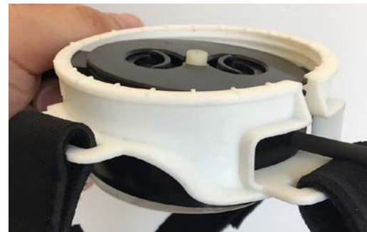
Figure 4C. Transducer and Transducer Holder showing clip mechanism in grooves to set angular position.
