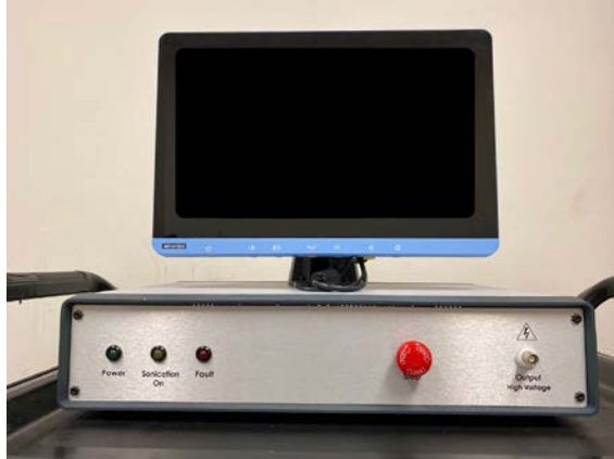
Figure 2a: Stimulator – Front. From left to right, the indicator lights include Power, Sonication On, and Fault. Large button is Emergency Shutdown. Connector on right is for the transducer cable.
