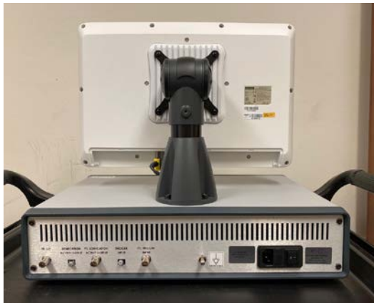
Figure 2b: Stimulator – Rear. From left to right, connectors include TTL I/O, Sonication Active Output (optical connection), TTL Sonication Active Output, Trigger Input (optical connection) and TTL Trigger Input. The master grounding pin is in the center. Connector on right is the power input module.
